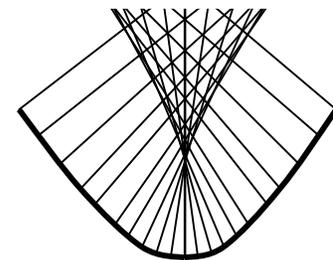
Following the ideas of She et al. [4], we designed a parabolic wave maker in order to generate waves that will focus in the Huygens cusp associated to the parabola. Figure 3 presents the ray pattern associated to waves propagating away from the parabola and that draws the cusp. Geometrical optics ray theory
