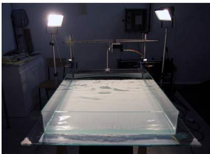
**Fig.4. The water table with its wave-maker and illuminating equipment.**
