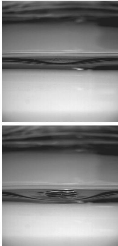
**Fig 5. Two consecutive snapshots of the breaking caused by the focusing of a solitary wave in a cusp.**
